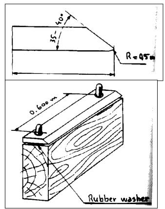
When you make the fold, the edges of the guard plates being in contact with each other, there will be a slight slippage of the piece with respect to either Assembly A or Assembly B. In order to eliminate any uncertainty, proceed so that any slippage takes place in assembly B by
