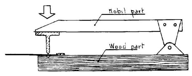
Another variety of folder can be made by the Amateur. Its operation is simpler than that of the folder described above: on the other hand it is difficult to fold other than a predetermined angle. It would be, however, very practical for making right angle folds which are the most common. Its principal elements are shown above and on the next page.
