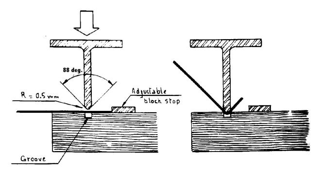
The matrix is composed of a groove  $2 \times 2$ or  $3 \times 3 \text{ mm}$  (0.079" to 0.112" or roughly 3/32") made in a wooden board (hard, if possible) perpendicular to the grain, and the punch is the web of a T-Bar, sharpened to 88° (for right angle folds) and with a radius of 0.5mm (.020").
