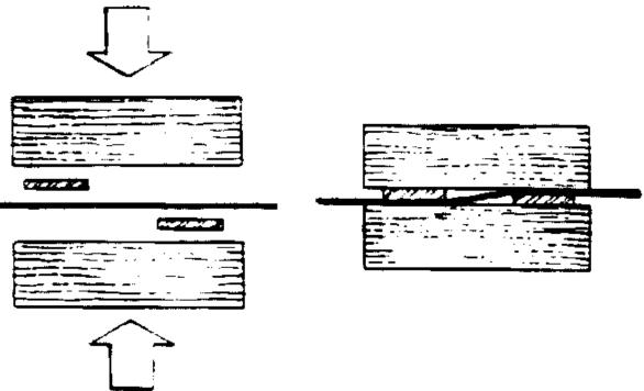
The thickness of the shims should be slightly greater than the depth of the offset (rise).
