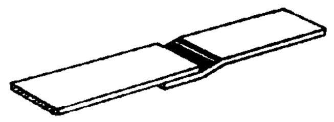
In the case of a strip of metal or of a relatively narrow part, the offset can be made simply by clamping the part between two staggered shims.
